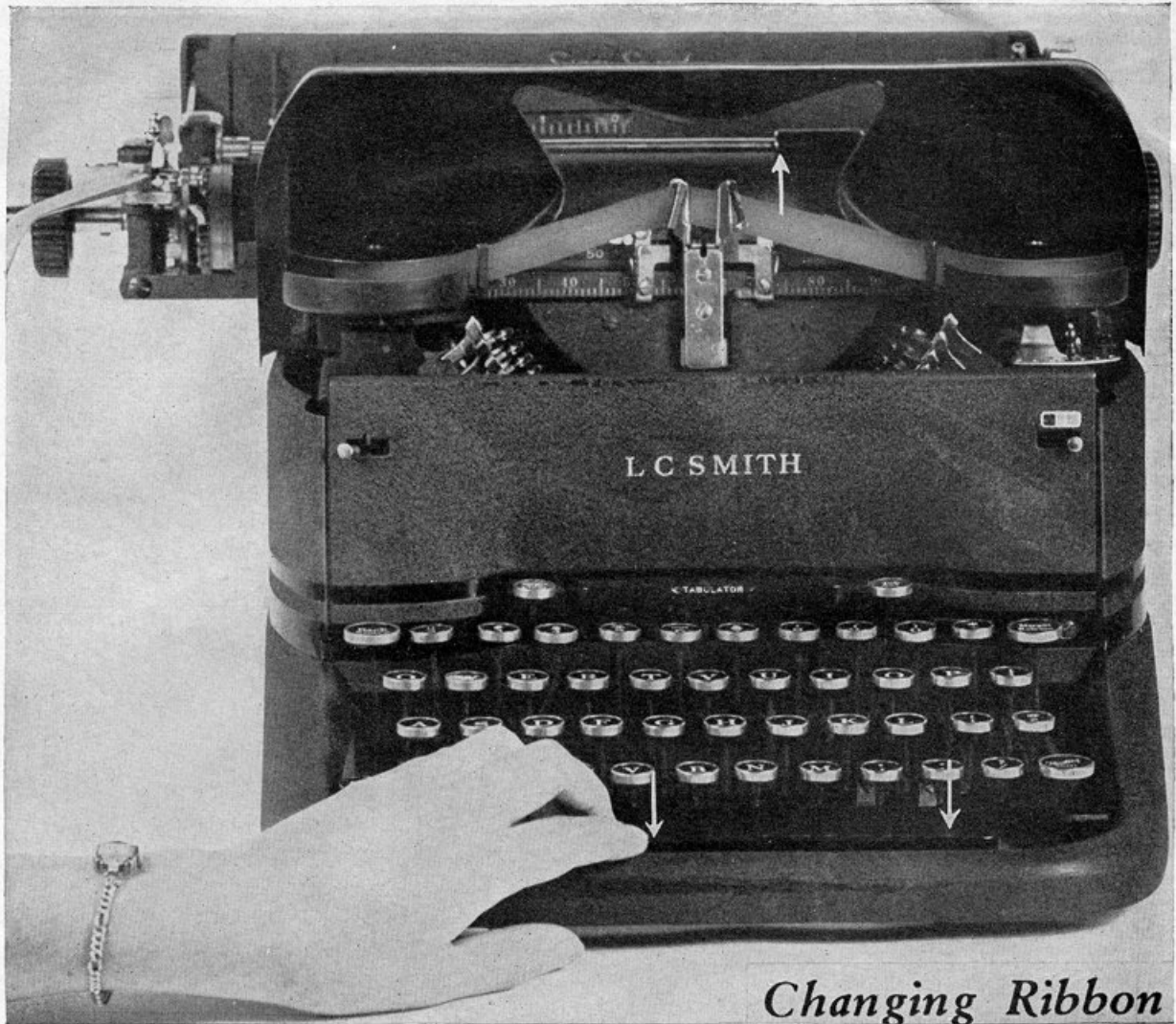
Figure 14.—Holding down space bar on L. C. Smith to raise ribbon for changing.
