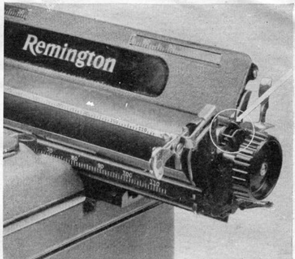
Figure 29.—Platen lock lever, locked, Remington Standard.
