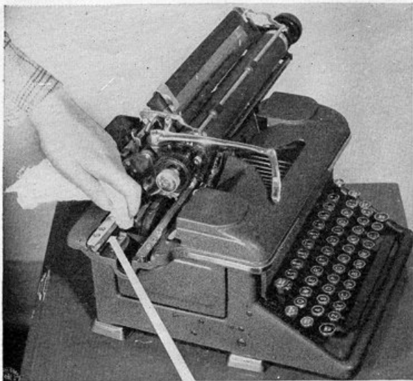
Figure 7.—Fixed carriage rail on standard typewriters.
