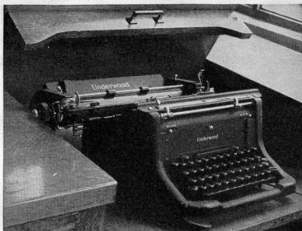
Figure 35.—Closing desk with typewriter carriage uncentered may bend platen end or break carriage frame.
